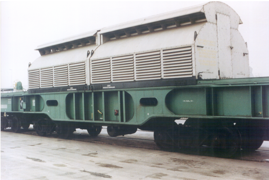
Wagon equipped with sliding canopies for the transport of irradiated fuels
