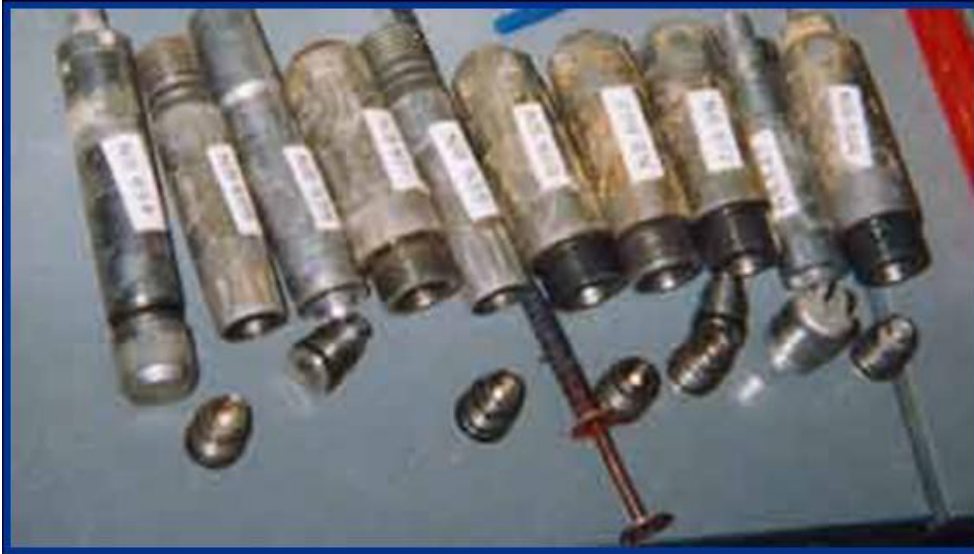
FIG 1. Examples of the ^{241}\text{Am} well-logging sources recovered by OSRP in the U.S.
