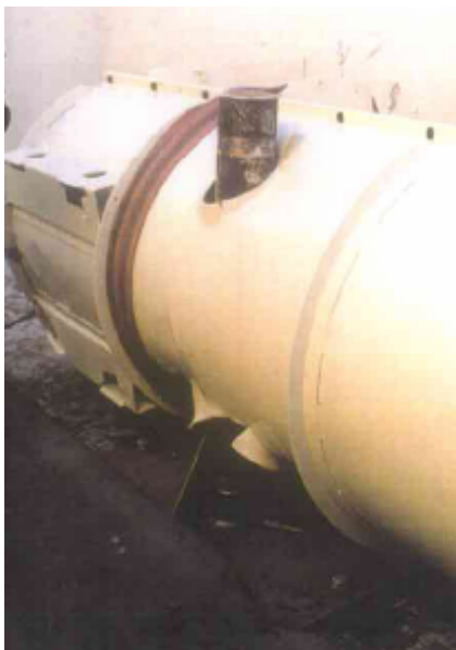
Double-perforation of a prototype of package by the regulatory punch (Courtesy of Framatome)
