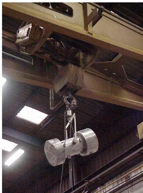
Position of drop with slap down (Courtesy of CEA)
